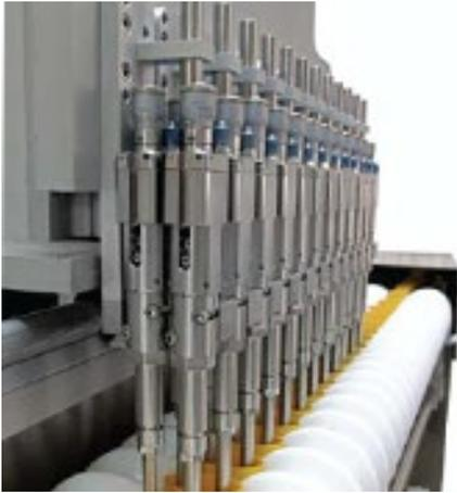
Provision for Servo Motor Controlled Bottom/Up Fill Motion for high viscosity products or foamy products.
