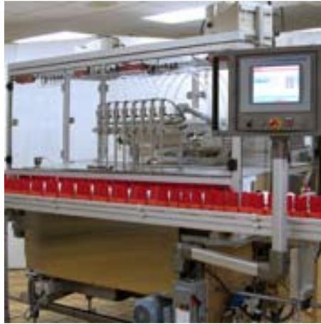
Heated Filling Systems are available, utilizing sealed heated chambers or electronic cartridge heaters.
