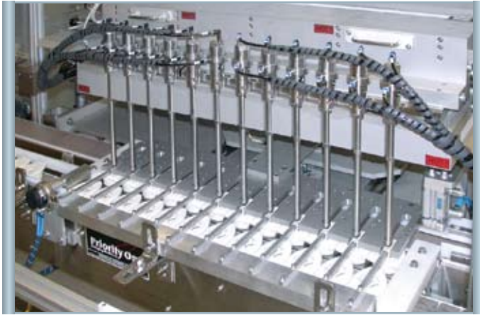
Heated Filler with Cross Push Container Indexing System
